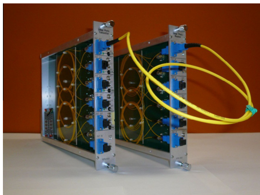
Fig. 22. Photograph of the optical transmitter and receiver NIM modules.
